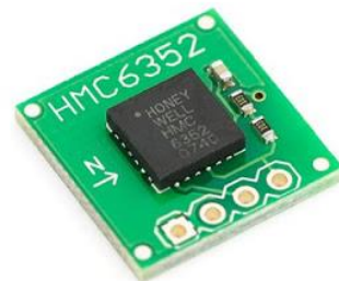
Gambar 2.6 Sensor Kompas Sumber : http://1.bp.blogspot.com/-W_K53jfTRIQ/ULSONg4BQ1I/AAAAAAAAAAU/fhPKWb_hqu4/s320/Sensor-Kompas-HMC6352.jpg
