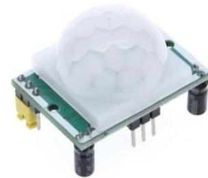
Gambar 5. HC-SR501 Passive Infrared Sensor (Anonim 2, 2024)
