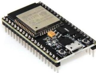
Gambar 4. Microcontroller Esp32 (Anonim 1, 2024)
