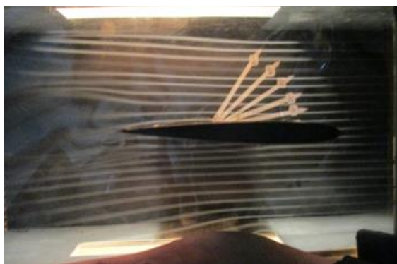
Gambar 4.3 Model Airfoil Simetrikal Posisi 0^\circ
