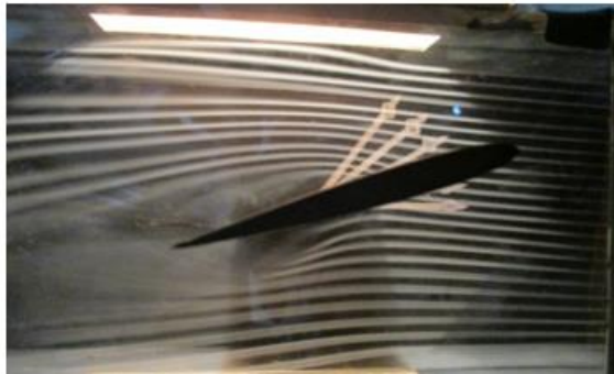
Gambar 4.6 Model Airfoil Simetrikal Posisi 20°
