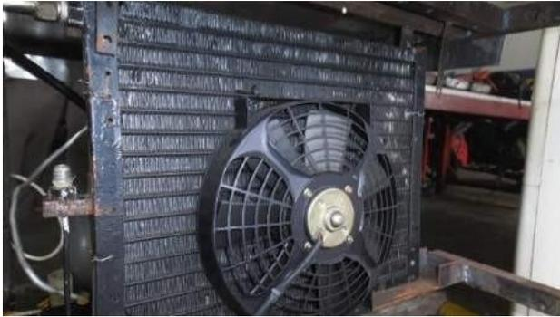
Gambar 3.3 Kondensor AC mobil
