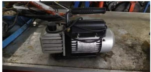
Gambar 3.6 Pompa Vakum
