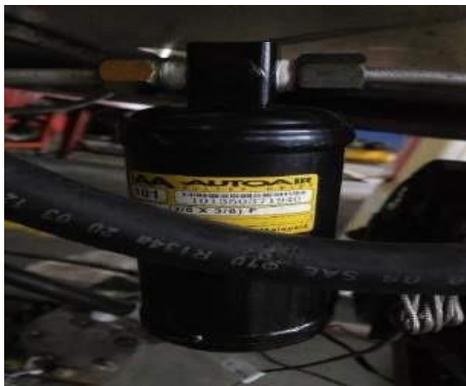
Gambar 3.8 Receiver dryer
