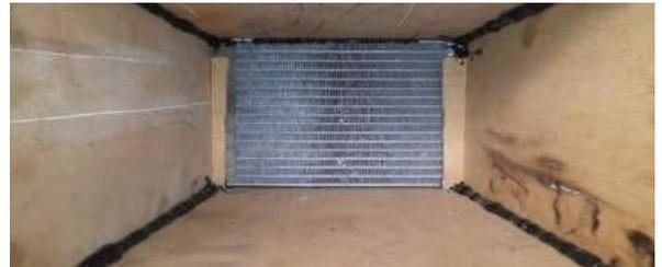
Gambar 3.5 Evaporator AC mobil
