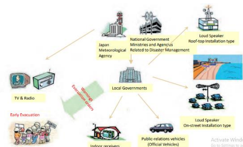
Gambar 8. Sistem Peringatan Dini di Jepang (Sumber: Cabinet Office, Disaster Management in Japan dalam Mukhlisin, 2024)
